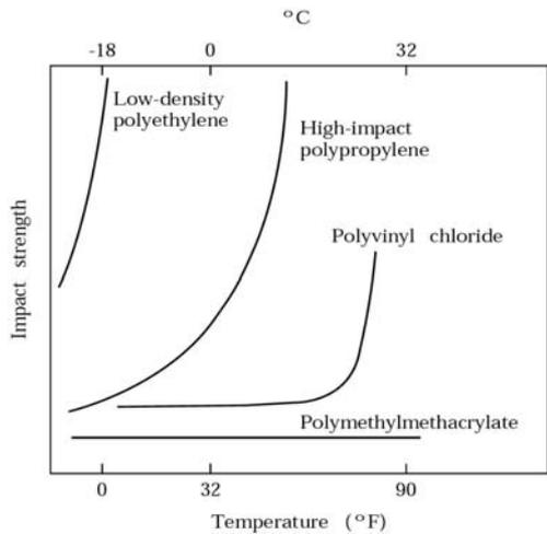
Effect of temperature on the impact strength of various plastics. Small changes in temperature can have a significant effect on impact strength.
