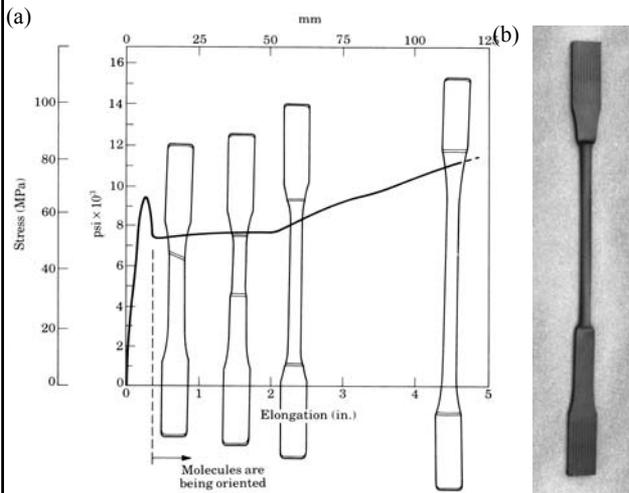
(a) Load-elongation curve, that shows *visco-elastic plastic behavior*, for polycarbonate, a thermoplastic. (b) High-density polyethylene tensile-test specimen, showing uniform elongation (the long, narrow region in the specimen).
