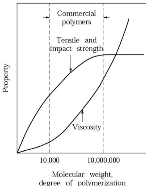
Effect of molecular weight and degree of polymerization (size of molecules) on the strength and viscosity of polymers. Molecular weight have a strong influence on the properties of polymers on mechanical and rheological characteristics
