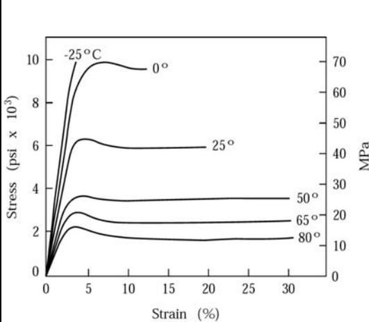
Effect of temperature on the stress-strain curve for cellulose acetate, a thermoplastic. Note the large drop in strength and the large increase in ductility with a relatively small increase in temperature.
