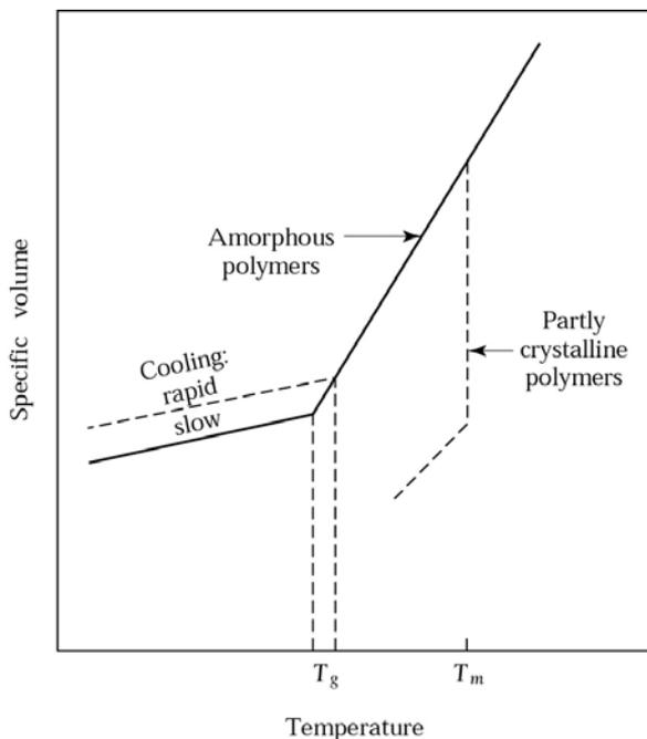
Specific volume of polymers as a function of temperature. Amorphous polymers, such as acrylic and polycarbonate, have a glass-transition temperature,  $T_g$ , but do not have a specific melting point,  $T_m$ . Partly crystalline polymers, such as polyethylene and nylons, contract sharply while passing through their melting temperatures during cooling.
