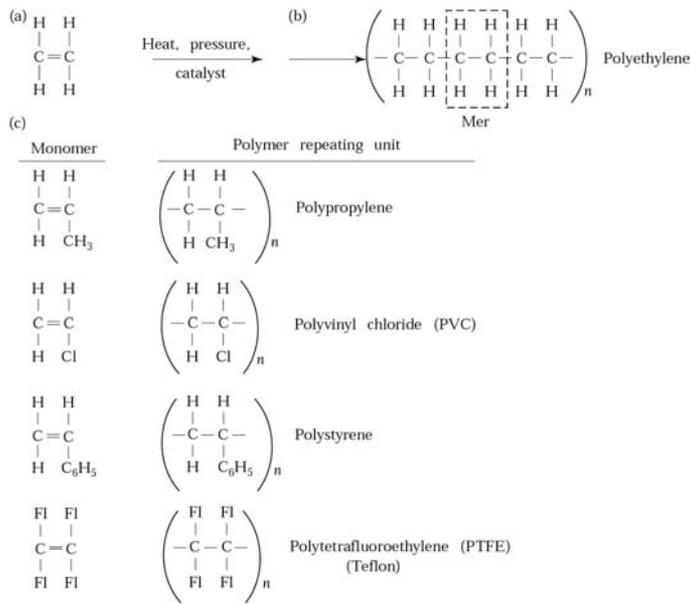
Basic structure of polymer molecules: (a) ethylene molecule; (b) polyethylene, a linear chain of many ethylene molecules; molecular structure of various polymers. These are examples of the basic building blocks for plastics
