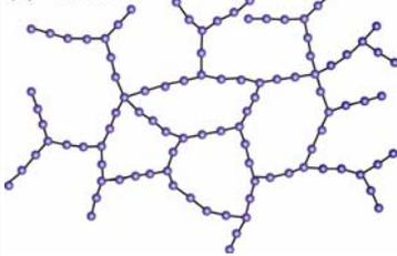
Schematic illustration of polymer chains. (a) Linear structure; thermoplastics such as acrylics, nylons, polyethylene, and polyvinyl chloride have linear structures. (b) Branched structure, such as in polyethylene. (c) Cross-linked structure-many rubbers or elastomers have this structure, and the vulcanization of rubber produces this structure. (d) Network structure, which is basically highly cross-linked--examples are thermosetting plastics, such as epoxies and phenolics.
