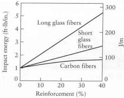
The properties of reinforced plastics are influenced by several factors. The most important are: type and shape of reinforcing material; the length of the fiber (short fiber are less effective than long); and the volume fraction of the reinforcing material. Another critical factor in reinforced plastic is the kind of bond between fiber and matrix.
