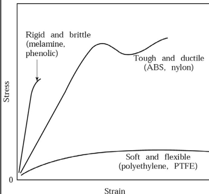
Typical stress-strain curves for some thermoplastics and thermosets at room temperature. Note that these plastics exhibit different behaviour: rigid, ductile, flexible. Plastics, as metals, undergo fatigue and creep phenomena as well.
