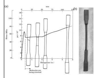
(a) Load-elongation curve, that shows visco-elastic plastic *behavior*, for polycarbonate, a thermoplastic. (b) High-density polyethylene tensile-test specimen, showing uniform elongation (the long, narrow region in the specimen).
